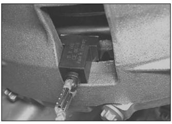
**Vehicles with automatic transmission:**Block crankshaft with special tool ZF1004
