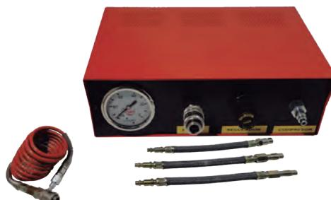
**Extractores de la bomba inyectora - Set tools for removing injection pump****US-953/1 [BMW-330]**
