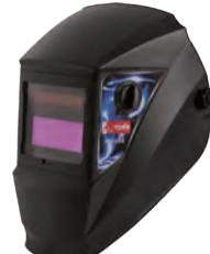
Automatic helmet mask ideal for TIG, MIG-MAG and MMA welding with external darkening adjustment (DIN 4/5 ÷ 9/9+13). The LCD liquid crystal filter automatically darkens when the welding arc is running and quickly returns to its transparent status when the arc is switched off. Light and comfortable to wear. Adjustable automatic darkening filter. Dark-light delay adjuster. Solar cell powered. Transparent glass protection filter.
